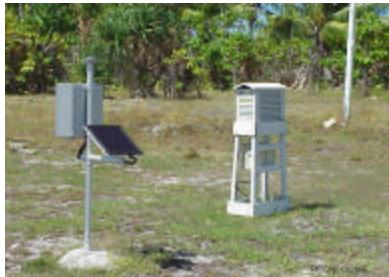
• Figure 19 A solar powered Automatic Weather Station
