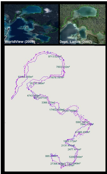
Figure 21: Outcome of using overlays and Liscad package. 21 mangrove Polygons (31.2 ha of mangrove vegetation)
