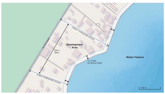
Figure 4: Diagram demonstrating required buffer between water features and new development and minimum provision for public access to foreshore.
